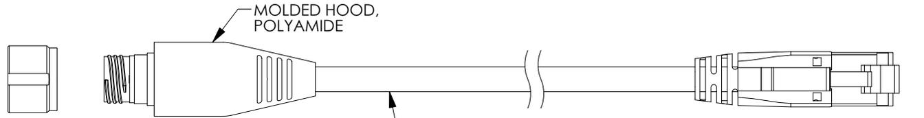
FOUR TWISTED PAIR, 26 AWG (7X34) STRANDED COPPER
