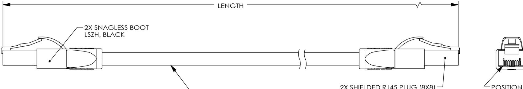
SHIELDED, FOUR TWISTED PAIR, CAT 5E MODULAR CABLE
