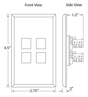
Note: QuickPort snap-in modules (connectors and bulkhead connectors and couplings) are sold separately. Please refer to the QuickPort module spec sheets for ordering information.
