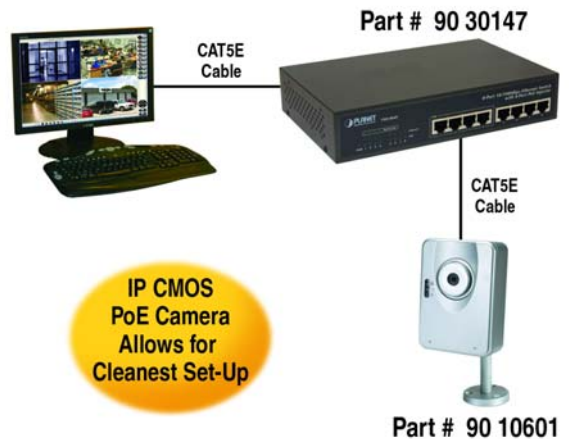
Diagram of IP CMOS PoE Camera Installation
