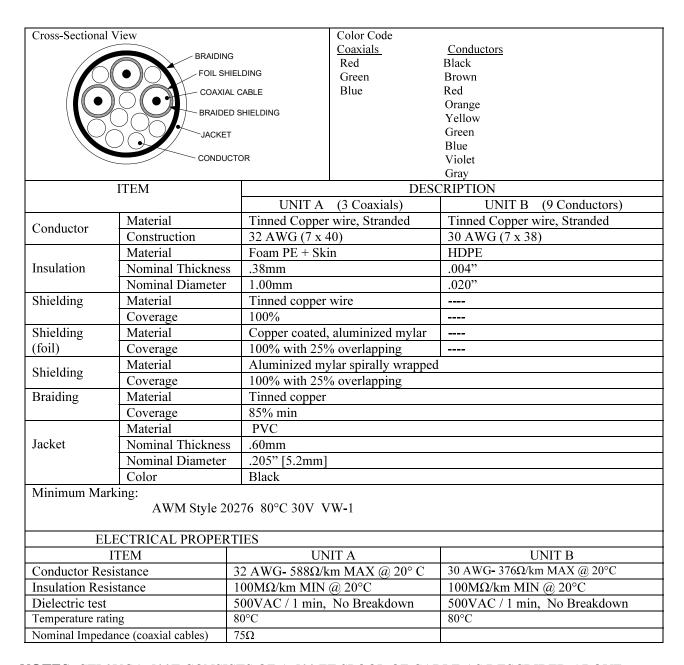
**NOTES**: CTL3VGA-500T CONSISTS OF A 500 FT SPOOL OF CABLE AS DESCRIBED ABOVE. TOTAL CABLE LENGTH TOLERANCE: +5% / -0%
