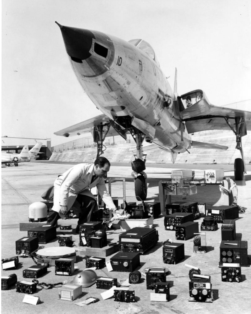
Caption: F-105 Thunderchief with LRUs laid out. Federated architectures mitigated the amount of wiring between discrete components and streamlined aircraft controls.
